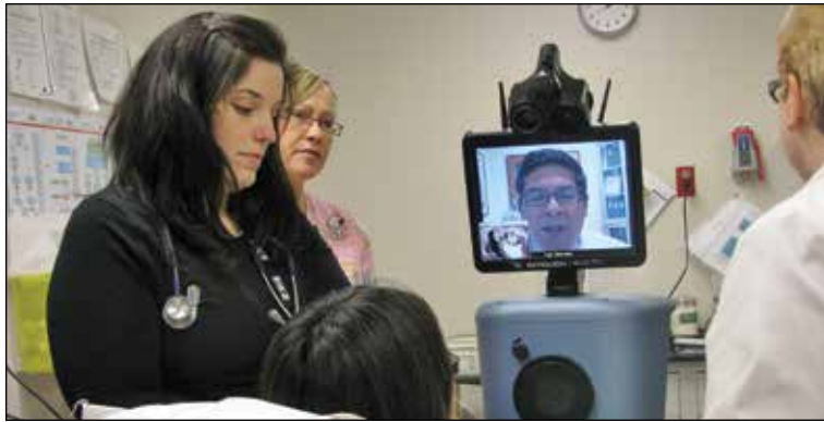
Dr. Mendez is seen on the video monitor of a remote presence robot at a patient's bedside
